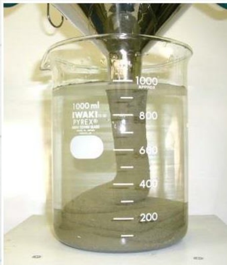
PRETASCON TYPE-AP anti-washout property in water
