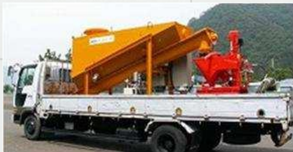
System equipped with hopper and feeder for dry mortar
